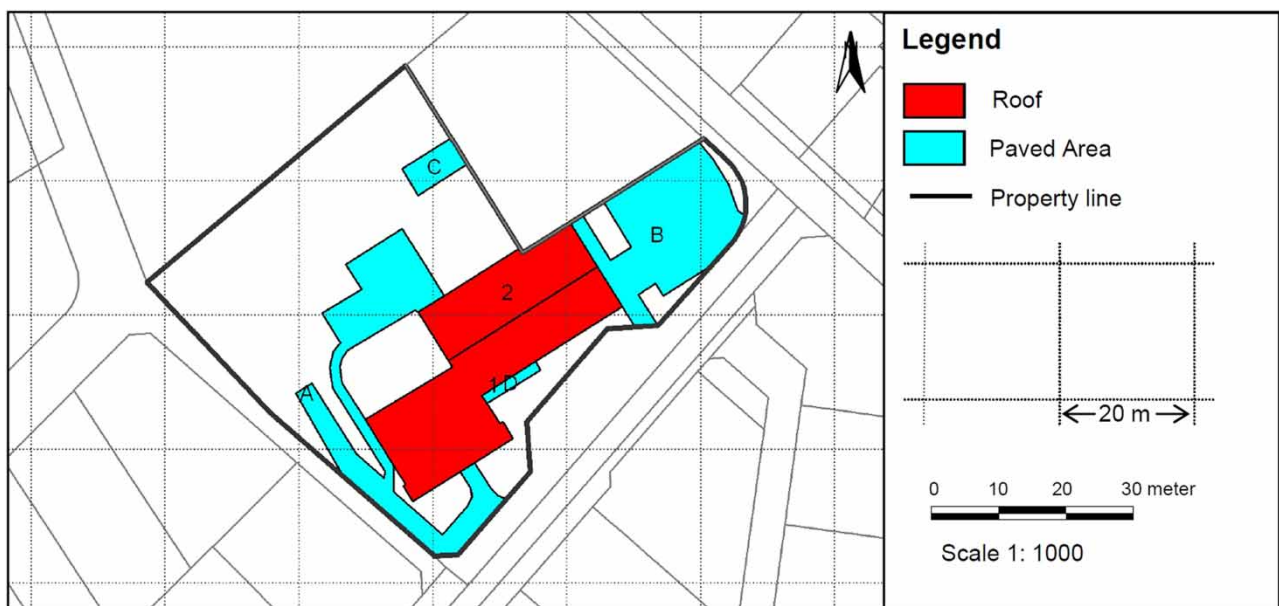
Figure 4 | Detail of an exemplary data entry form for verification of surface drainage situation at property level.
